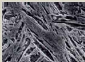
This microstructure differs from the rough acicular lamellar structure which is typical of the fully martensite steels (conventional 500 HB water quenched steels).
