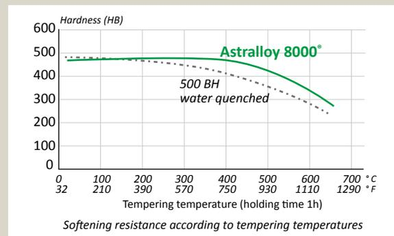
It is also possible to process the steel at high temperatures 500° – 550°C (930° – 1020° F) (hot forming: bending, rolling) followed by a slow air cooling without inducing any significant drop of hardness (about 30 – 50 HB).
