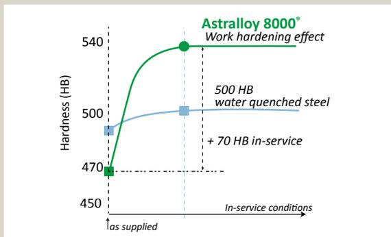
In addition, the advanced ductility of the retained austenite contributes to the improved in-service lifetime by allowing larger micro shearing which delays the ultimate tearing of metal particles from the surface of the material exposed to the abrasive.
