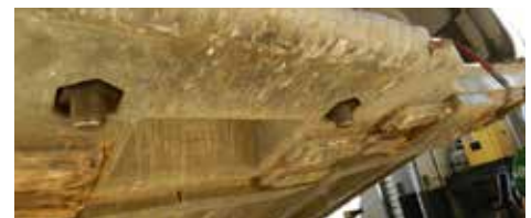
Dutchman block with the two bolts holding Astralloy’s insert in place. The Dutchman “latch” slides through the hole and catches on our AV insert.
